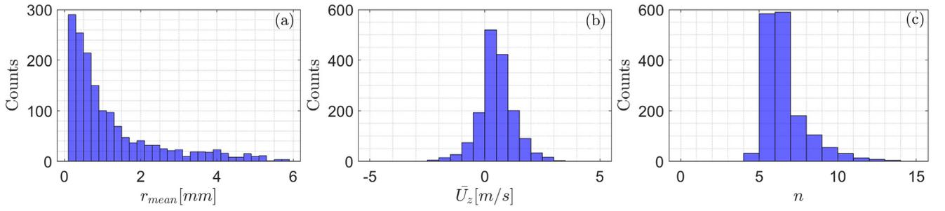
Fig. 15. Histograms of (a) mean pocket radii ( $r_{mean}$ ), (b) mean out-of-plane velocities inside pockets, and (c) maximum value of  $n_{max}$  used.
