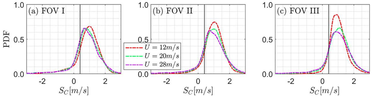
**Fig. 1.** PDFs of reactant pocket consumption speeds in field of view (FOV) (a) I, (b) II, and (c) III for single Bunsen flames. Vertical lines represent  $s_L=0.4$  m/s.
