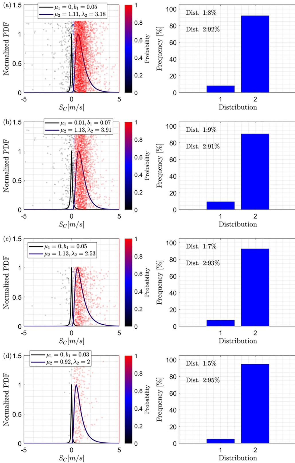
**Fig. 19.** Mixture-model results of out-of-plane consumption rate PDFs from measured PDFs for (a) all pockets, (b) pockets with  $0 \text{ mm} < r_{\text{mean}} \leq 2 \text{ mm}$ , (c) pockets with  $2 \text{ mm} < r_{\text{mean}} \leq 4 \text{ mm}$  and (d) pockets with  $r_{\text{mean}} > 4 \text{ mm}$ . (For interpretation of the references to color in this figure, the reader is referred to the web version of this article.)
