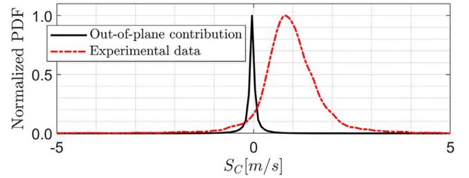
**Fig. 13.** Out-of-plane consumption rate PDF for 3D pockets (solid black line).
