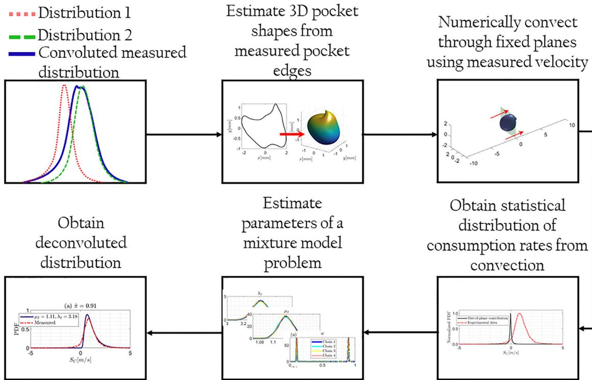
Fig. 8. Flowchart of the framework for obtaining true consumption rates from measured consumption rates.
