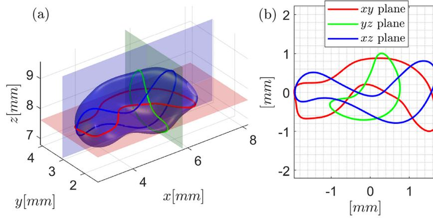
Fig. 4. (a) Flame pocket shape in 3D and (b) planar cuts of the pocket along the  $xy$ ,  $yz$ , and  $xz$  planes at the centroid location of the pocket.
