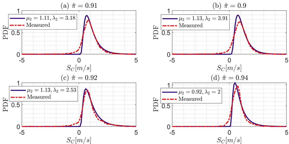
**Fig. 20.** Comparisons between corrected and measured PDFs for (a) all pockets, (b) pockets with  $0 \text{ mm} < r_{\text{mean}} \leq 2 \text{ mm}$ , (c) pockets with  $2 \text{ mm} < r_{\text{mean}} \leq 4 \text{ mm}$  and (d) pockets with  $r_{\text{mean}} > 4 \text{ mm}$ .
