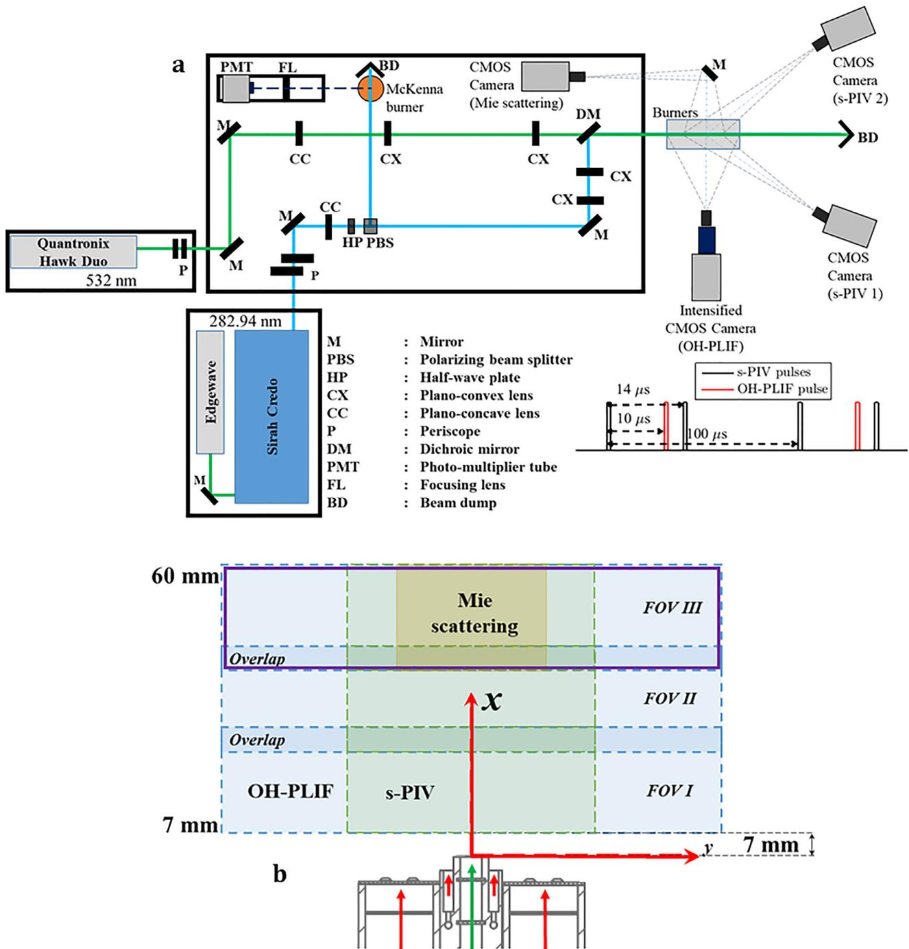
**Fig. 6.** (a) Laser optical setup and (b) measurement locations with respect to the burner exit location. In sub-figure (b), the red arrows correspond to the flow for the back-support and anchoring pilot flames and the green arrow corresponds to the flow for the main flame. (For interpretation of the references to color in this figure legend, the reader is referred to the web version of this article.)
