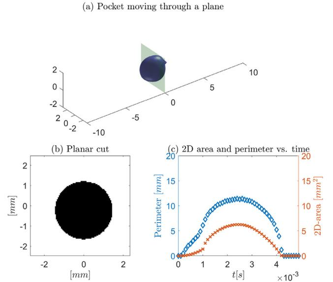
**Fig. 12.** (a) Convection of 3D pocket through  $(x, y, 0)$  plane, (b) cross-section pocket contour, and (c) time-series of cross-section area and perimeter; video provided in Supplementary material.
