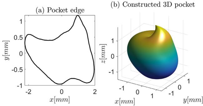
**Fig. 11.** (a) Flame pocket edge and (b) constructed 3D pocket.
