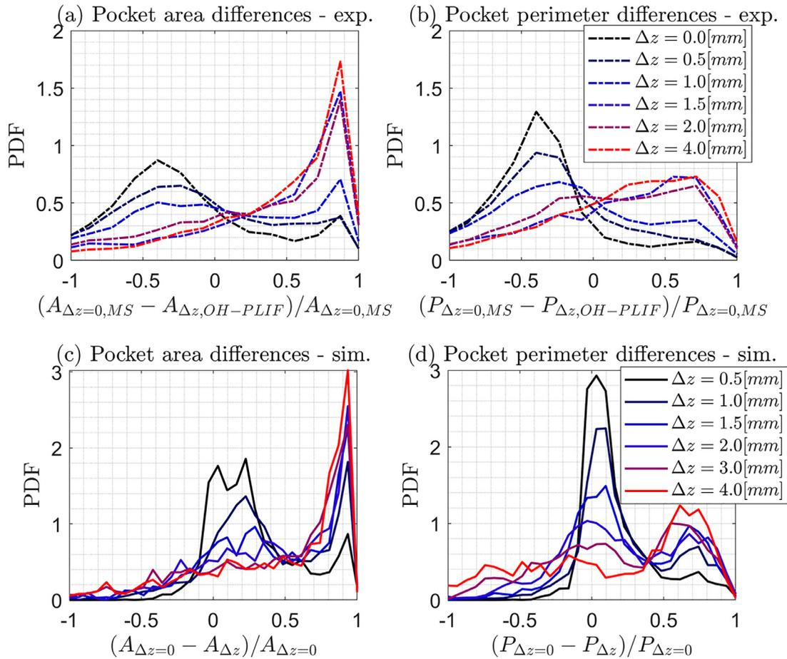
**Fig. 14.** Relative differences in experimentally measured pocket (a) areas and (b) perimeters for different plane offset values. Relative differences in constructed 3D pockets: (c) areas and (d) perimeters for different slices.
