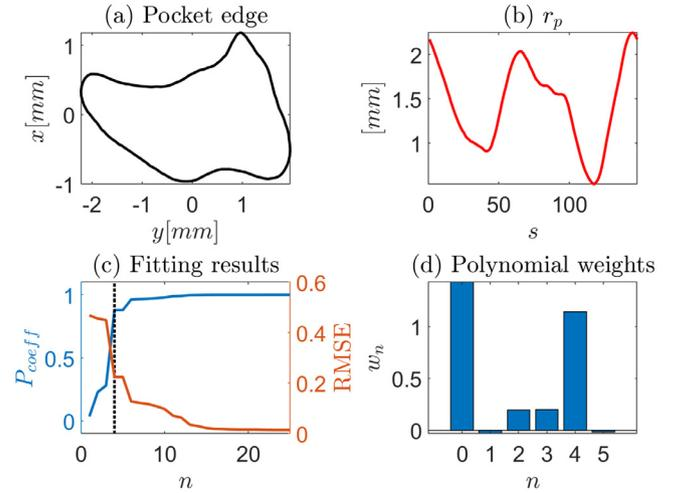
Fig. 9. (a) Centered flame edge, (b) value of  $r_p$  along flame edge, (c)  $P_{coeff}$  and RMSE, and (d)  $w_n$  for fitting with a maximum polynomial order of 7.
