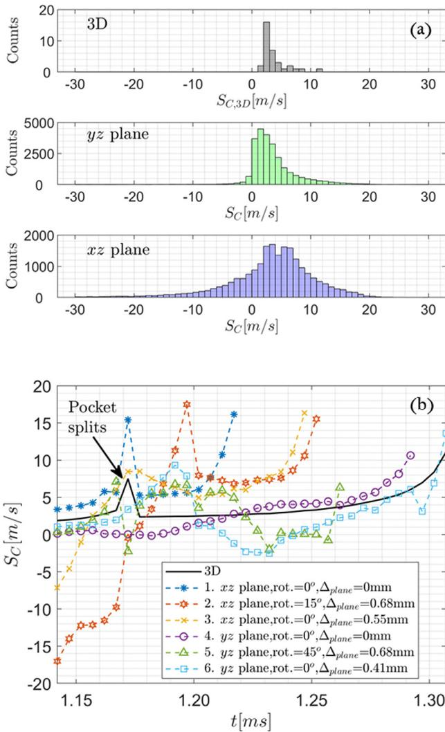
Fig. 5. 2D pocket consumption rate (a) histograms and (b) time series.
